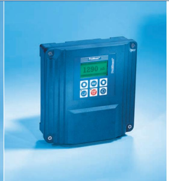
Up to four cooling circuits or boilers can be controlled simultaneously by the AQUATRAC® cooling tower control. It can perform all the requisite functions, including bleed control, metering of two biocides and inhibitors, as well as monitoring of the entire process. Cooling tower control can be performed in conductive or volumetric mode.
